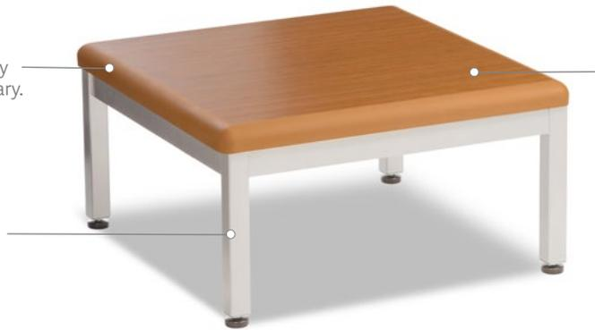
Decorative high pressure laminate is permanently bonded to a core of 45 lb density particle board with permanently embedded T-nuts for securing top to base.
